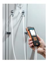
With the testo 440 dP model, which includes a differential pressure sensor, you can ensure that the filters in air conditioning systems are working properly and no contamination in the outdoor air contamination gets indoors.
